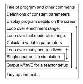
Figure 4 : General structure of the infinite reactor simulator
