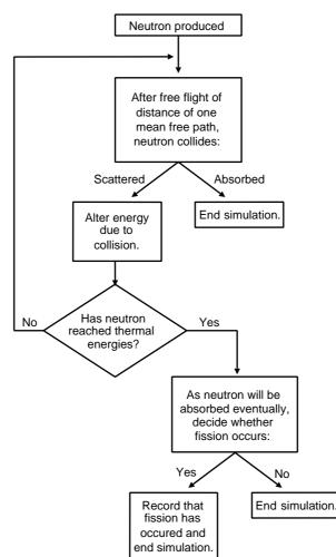
Figure 3 : Flow chart for infinite reactor simulation:
